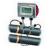
Mobile flow meter to locate leaks -> available on loan from the Watsan Technical Referent
