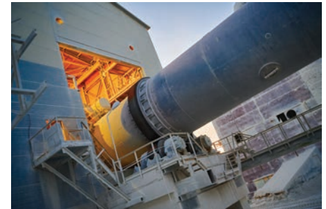
Cement factory rotary furnace at +/- 1450°C
